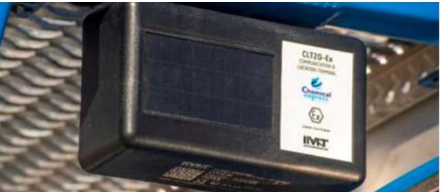
Solar-powered tracking and localization device
