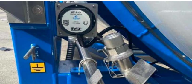
Environmental monitoring sensor installed on tank containers
