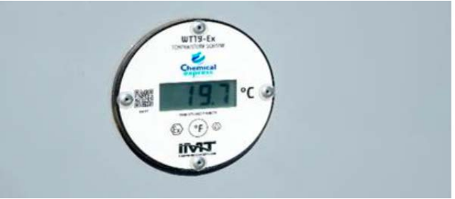
Digital thermometer for detecting the internal temperature of the container
